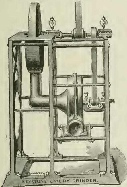
but extra powerful exhauster, which takes its driving-power direct from the mandrel of the grinder, thus combining the two tools in one—a saving in first cost of construction to the consumer of at least fifty per cent, as the usual countershaft, pulleys, belts, etc., are dispensed with, without taking into account the economy of space, which in itself is a desideratum.
