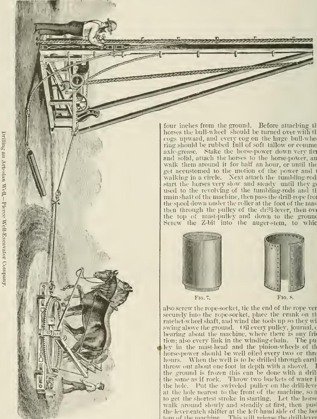
Drilling an Artesian Well—Pierce Well-Excavator Company.
