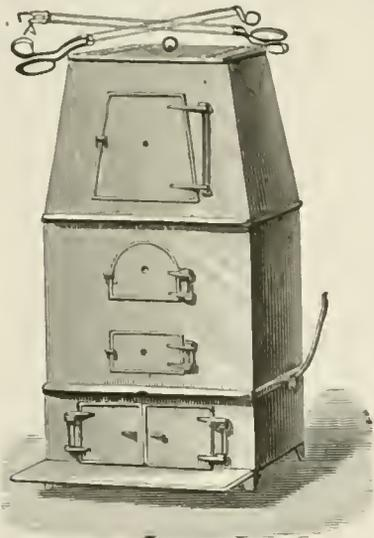
circulation of air over the contents. The ordinary muffle, closed at the back, can also be used as with any other furnace. The doors have small holes in them through which the reactions going on within the muffle may be watched without injury either to the operation or the operator.
