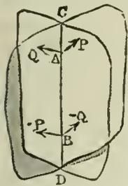
each end of this arm we shall have a pair of forces, say P and Q, inclined to one another at the angle of inclination of the planes. Their resultant, by the composition of forces, will be a force R, acting in a line between the planes. We shall have then forces R acting at each end of the arm, and evidently in directions parallel and opposite.  $R \times \text{arm } AB$ , then, is the moment of the resultant couple. Having seen how to com-
