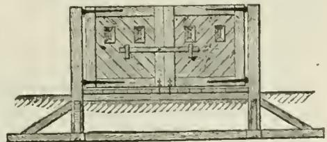
of all barriers should not be less than six feet above the ground. In the barriers with open leaves, the vertical pieces are usually extended from eighteen inches to two feet above the top rails, and their upper ends sharpened. In those which are solid, it is usual to arrange some obstruction upon the top rail, such as sharp-pointed spikes, broken glass, etc., to interfere with persons climbing over the top. It is usual
