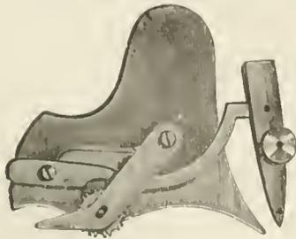
German-silver plate, upon which is fastened a pen connected by a small bar and a ratchet movement with a rolling wheel. The bar is kept in its place by a small spring. Extra wheels of different patterns accompany the instrument, which, being readily changed, allow the making of various forms of lines. In using the instrument, care should be taken that the small point behind the pen rests on the paper, as
