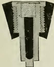
stock, which can, however, be used with the aid of an *adapting-ring* of gun-metal, which is serewed in to reduce the diameter of the hole to the proper dimensions. The 15-inch spherical shell are cast with three fuse-holes equally distant from each other, and situated in the angles of a triangle 4 inches apart. See *Fuse-hole* and *Shells*.
