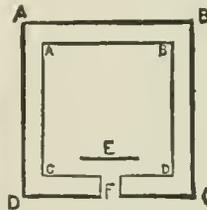
by  $x$  the number of yards in the side A B, the side A B will be equal to  $x$  diminished by twice the distance between A B and A B, which distance may be taken on an average at nine yards; the area of the square B C, or of the terre-plein, will then be represented by  $(x - 9)^2$ . Let the following notation be adopted:  $y$ , the number of the garrison;  $r$ , the reserve taken from the
