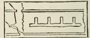
The first cut is made horizontally, and finished, which will be known by the earth falling through it; the vertical cuts are then made, there being one at each end of the intended breach. These cuts are commenced at the horizontal cut, and raised until the wall, isolated from its supports, sinks, overturns, and breaks into pieces, which become covered by falling earth. If the earth be sustained by its tenacity,
