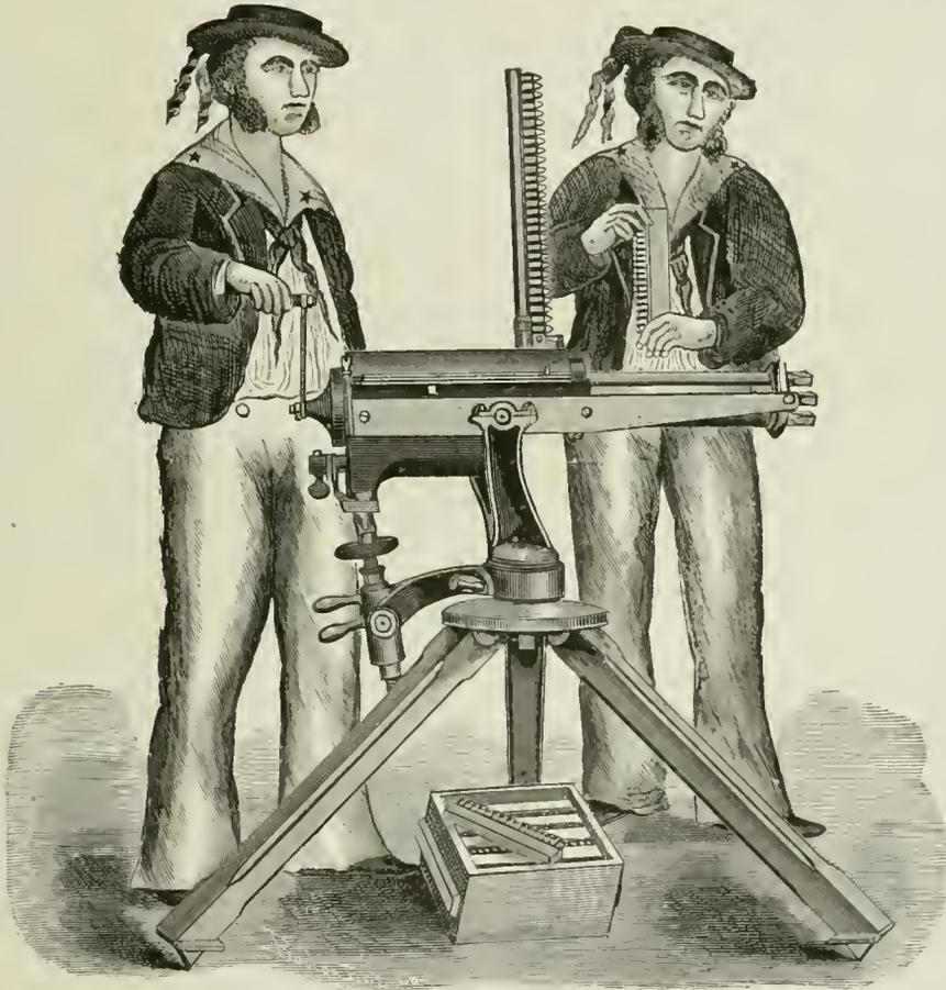
Lowell Battery-gun, mounted on Tripod.
