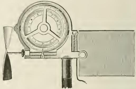
shows this instrument adapted for use in small rivers and streams, or to show the number of gallons flowing from any reservoir or vessel. The mean velocity
