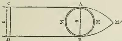
spherical-headed, elongated projectile of the same diameter represented by ACDBM, and moving with the same velocity, is 487 lbs., thus showing a difference of 68 lbs. total pressure. Now supposing the elongated projectile to move steadily, point first, the pressure on the respective heads, A, M, B, must be the same; therefore the difference of the total pressure,
